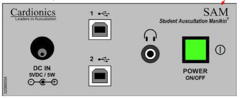
• The SAM II trainer is basically a USB speaker. Make sure to connect the SAM II torso to the laptop via USB before powering on the laptop.
